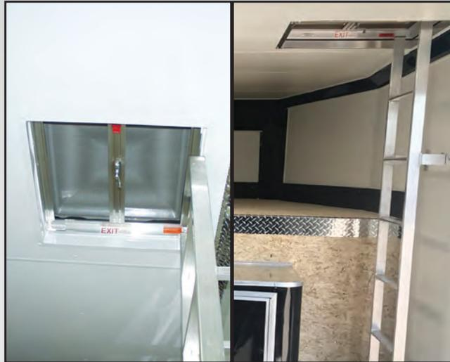
**ROOFTOP ESCAPE HATCH** - This escape hatch comes with a quick release push and optional aluminum ladder. The hatch also serves as a skylight and operable air vent.
