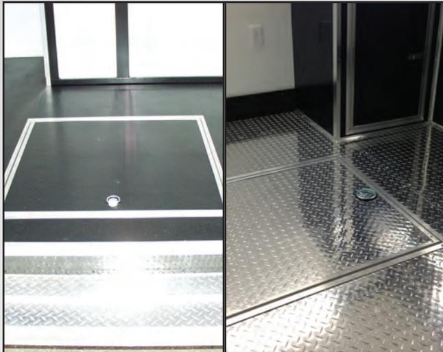
**RECESSED TIRE COMPARTMENT** - Large enough for a full-size spare trimmed to match trailer floor.
