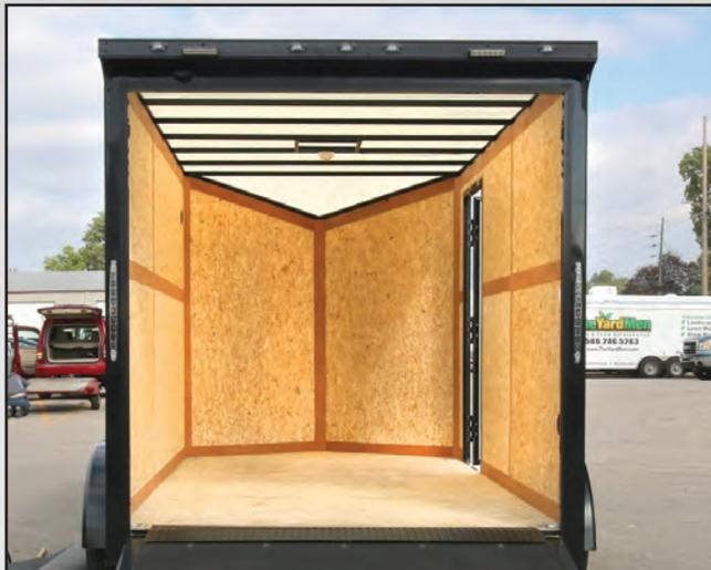
**TRANSLUCENT ROOFING**- An easy solution to light inside of the trailer during the working day—a common option for enclosed construction and landscape trailers.
