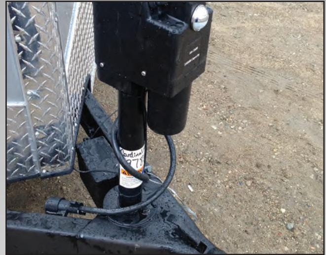
**12-VOLT POWERED TONGUE JACK** - This power jack makes hooking up to heavy-trailers as easy as the push of a button.
