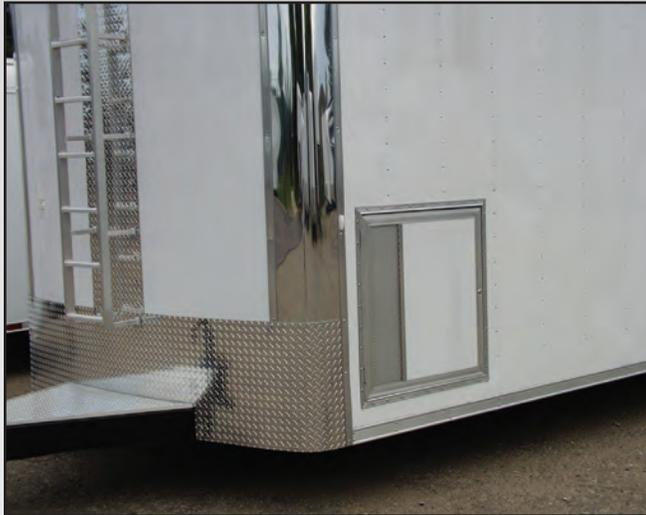
**GENERATOR DOORS** - Lockable generator doors give shelter and security for on-board power with ample ventilation.
