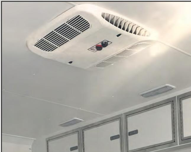
**ROOF AIR CONDITIONING** - This roof mounted air-conditioning unit has directional vents, variable temperature knob, and three-position cool and fan.
