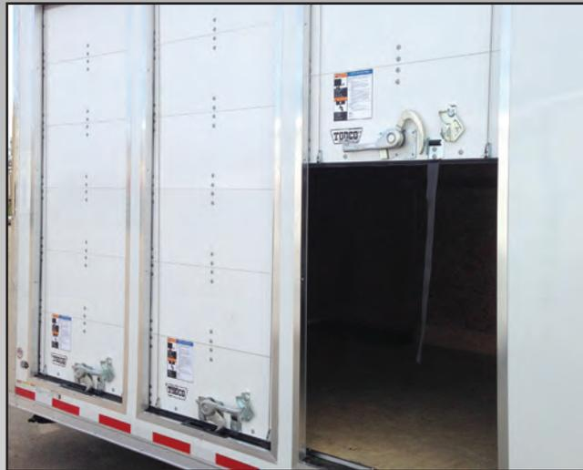
**ROLL UP DOOR** - This multi-panel, track-mounted roll-up door combines the ease of spring-assisted action, with Stealth construction and durability.
