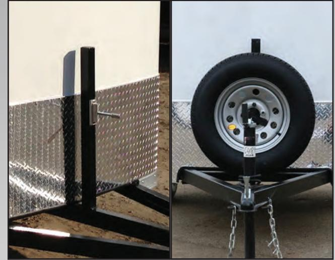
**SPARE TIRE MOUNT** - Always handy, this spare tire mount keeps a full sized tire ready for repair.
