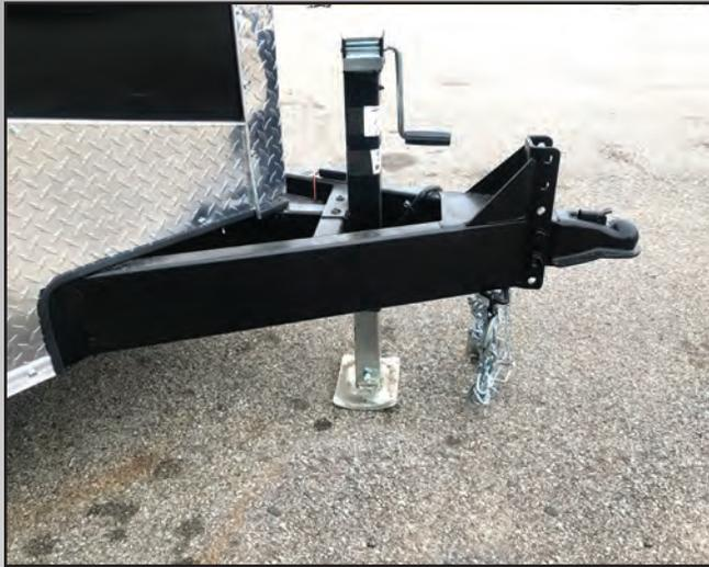
**HEAVY DUTY JACK** - This fixed-mount heavy duty jack is installed to take the maximum load on its oversized foot.
