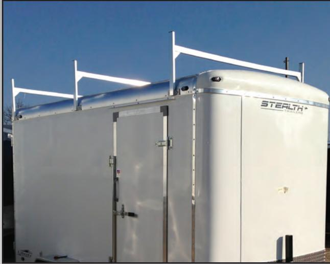
**ROOF LADDER RACK** - Welded, tubular aluminum ladder racks come in a variety of sizes to accommodate any size trailer or load.
